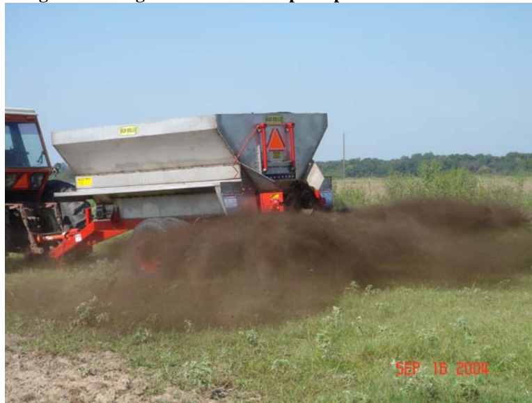
Figure 1. TWRI designed and High Roller built compost spreader for Fort Hood compost project.
